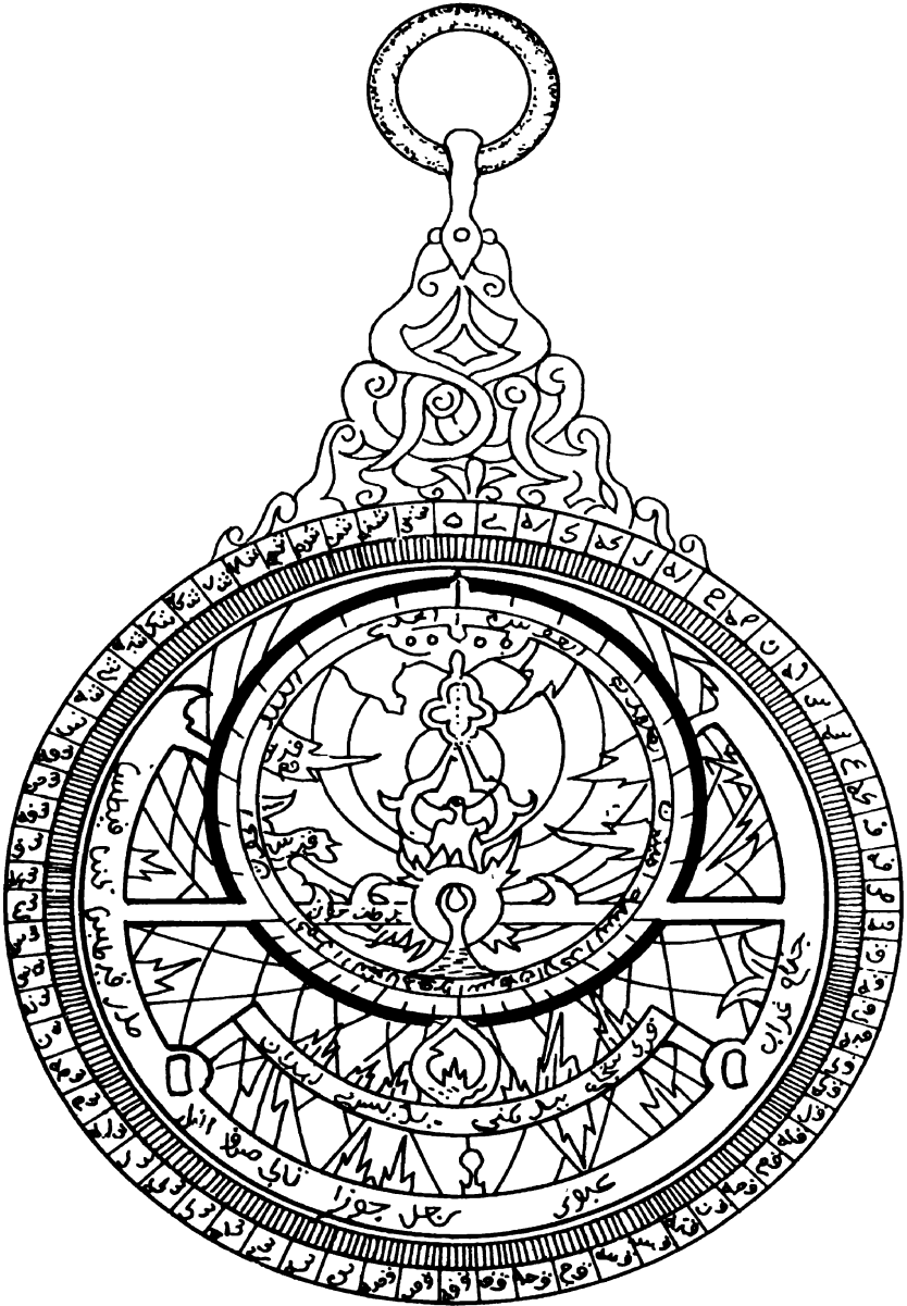
ASTROLABE : FRONT SHOWING THE SPIDER WITH STAR MAP AND PLATE FOR READING THEIR COORDINATES
